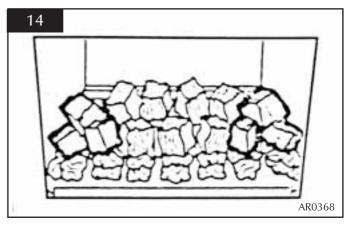
6.12 Place five small coals along the rear of the flame baffle, resting against the rear ledge, see diagram 15.
